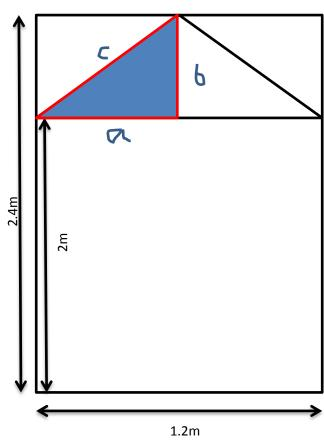
So we need 0.721m left from the clear polycarbonate sheet this is the minimum length for a roof panel.
